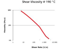
The above values were Calculated from data for 100 µm produced on a 75mm Barrnage extruder with 190°C melt temperature using a 2:1 blow ratio and a gap die of 3.0 mm.
